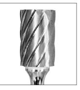
ALUMNA CUT For use on aluminum, magnesium, soft steel and nonferrous materials such as hard plastic, rubber and wood. Provides easy chip flow and faster stock removal with little or no clogging.
