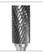
**DOUBLE CUT**Basically a standard cut tool, with cuts made on the left hand spiral. The design produces a finer finish on material and reduces the size of the chips and slivers. It gives greater tool control.
