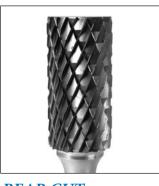
**BEAR CUT**Designed to substantially cut manufacturing production costs. This design and cut removes more material per hour. Engineered for heavy-duty applications. More durable due to the depth of the teeth. More resistant to chipping. Wider teeth make longer chips, which break up easier, and the profile of the teeth makes them less prone to filling up with chips.
